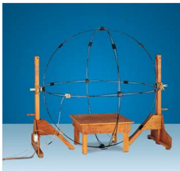
R&S® HM020 set up for measurement with antenna height reduced
